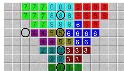
Figure 2: Weld Cross-Section (passes are numbered)
